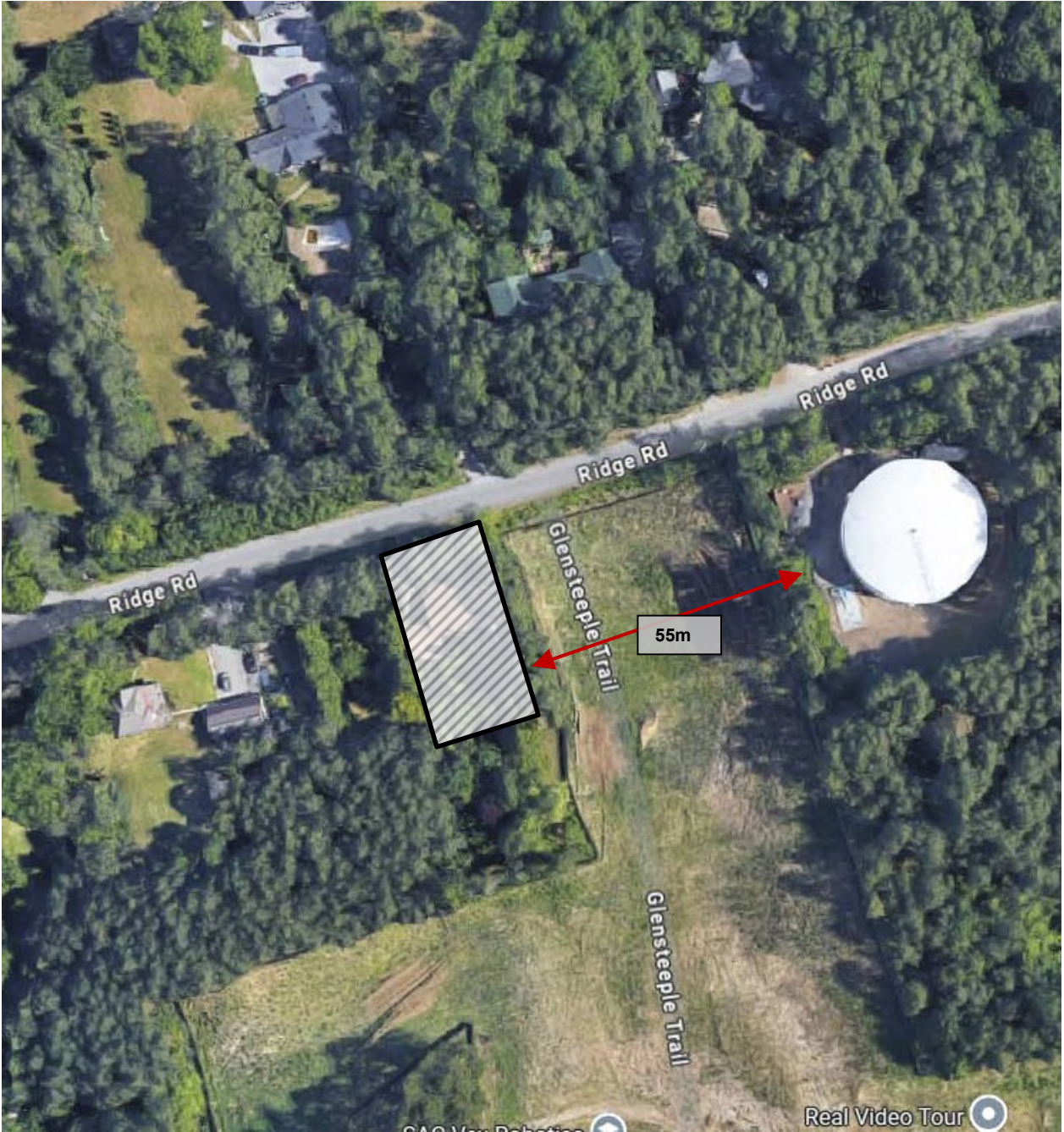
FIGURE 3 107 RIDGE ROAD – SITE PLAN DISTANCE FROM THE STATIONARY NOISE SOURCES
