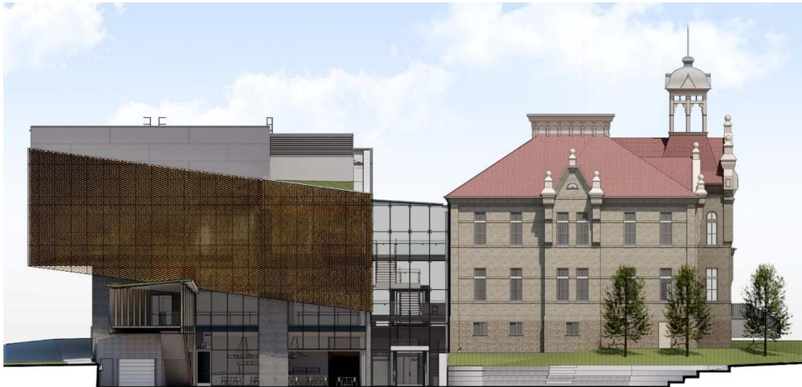
*Figure 1 - West Elevation with Bronze Anodized Aluminium*
