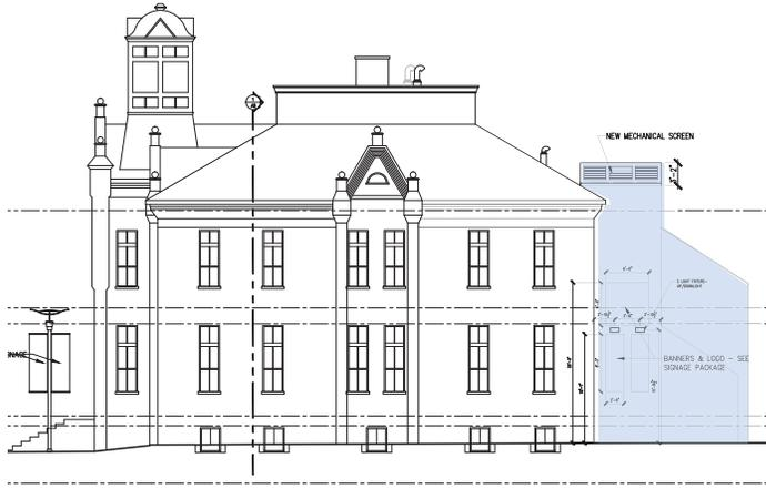
Existing east elevation, showing rear addition to be removed in blue (Lynch & Comisso; Annotated by ERA, 2018).
