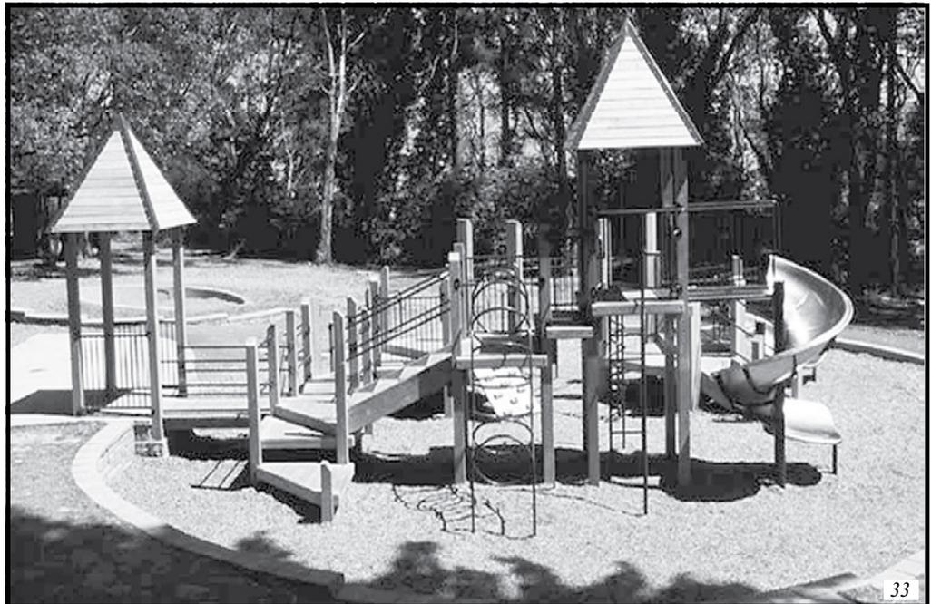
*Accessible surfaces can include impact-attenuating tiles made of recycled rubber and engineered wood fiber that meet the ASTM requirements for accessibility and safety. The design can be created so safety is not compromised for individuals using the playspace where both standards are applied.*
