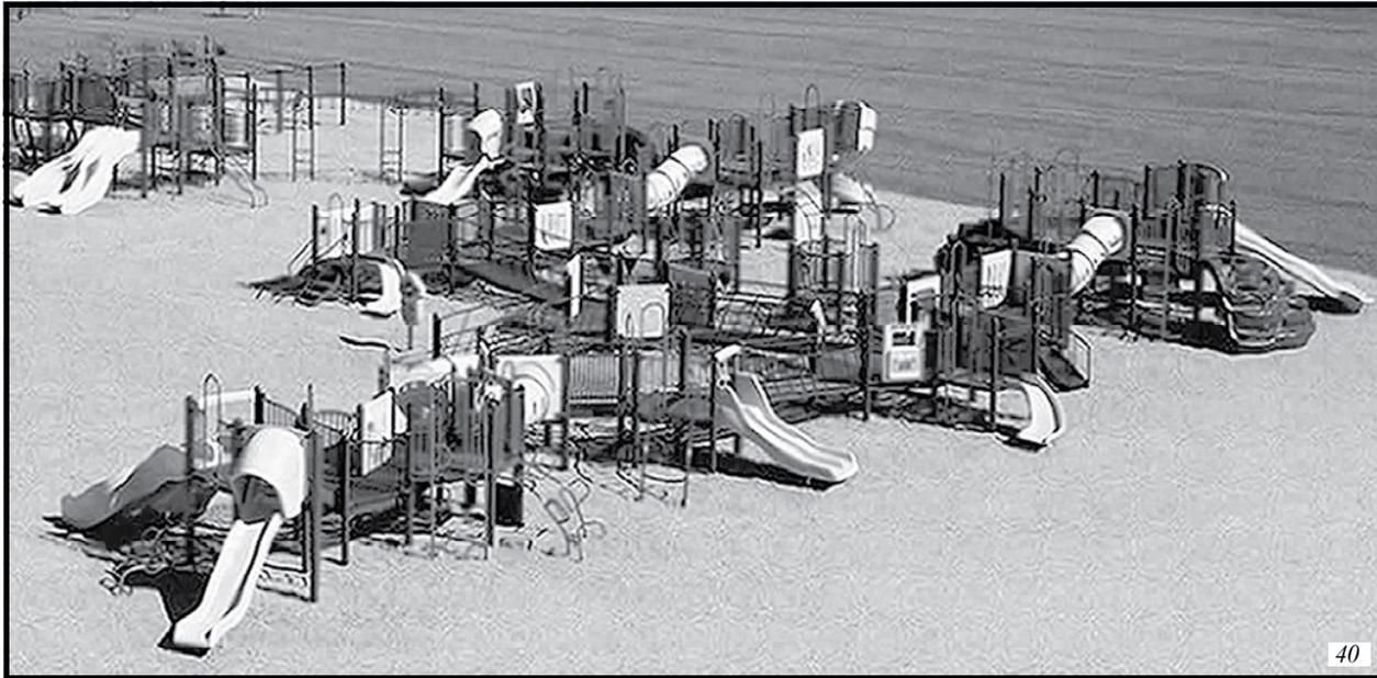
*This playspace has more than 20 play components and provides ramp access to elevated play components. The ramp system, consisting of ramp runs and landings, must connect at least 25 percent of the elevated play components. The balance of the elevated components required to be on an accessible route may be connected by the ramp system, or by a transfer system.*
