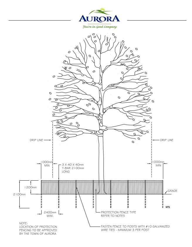
TYPE I PROTECTION FENCE PLASTIC MESH SAFETY FENCE OR WOOD SLAT SNOW FENCE
