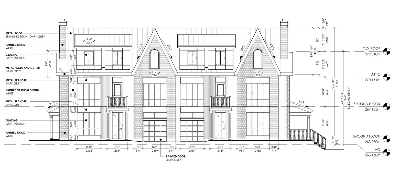
METAL ROOF STANDING SEAM - DARK GREY PAINTED BRICK T.O. ROOF 272.810m WHITE GLAZING **GREY MULLION** METAL FACIA AND GUTTER DARK GREY ATTIC 270.151m METAL SPANDREL DARK GREY METAL SPANDREL DARK GREY SECOND FLOOR 267.103m METAL ROOF STANDING SEAM - DARK GREY GLAZING -**GREY MULLION** PAINTED BRICK GROUND FLOOR 263.750m AG 263.160m
