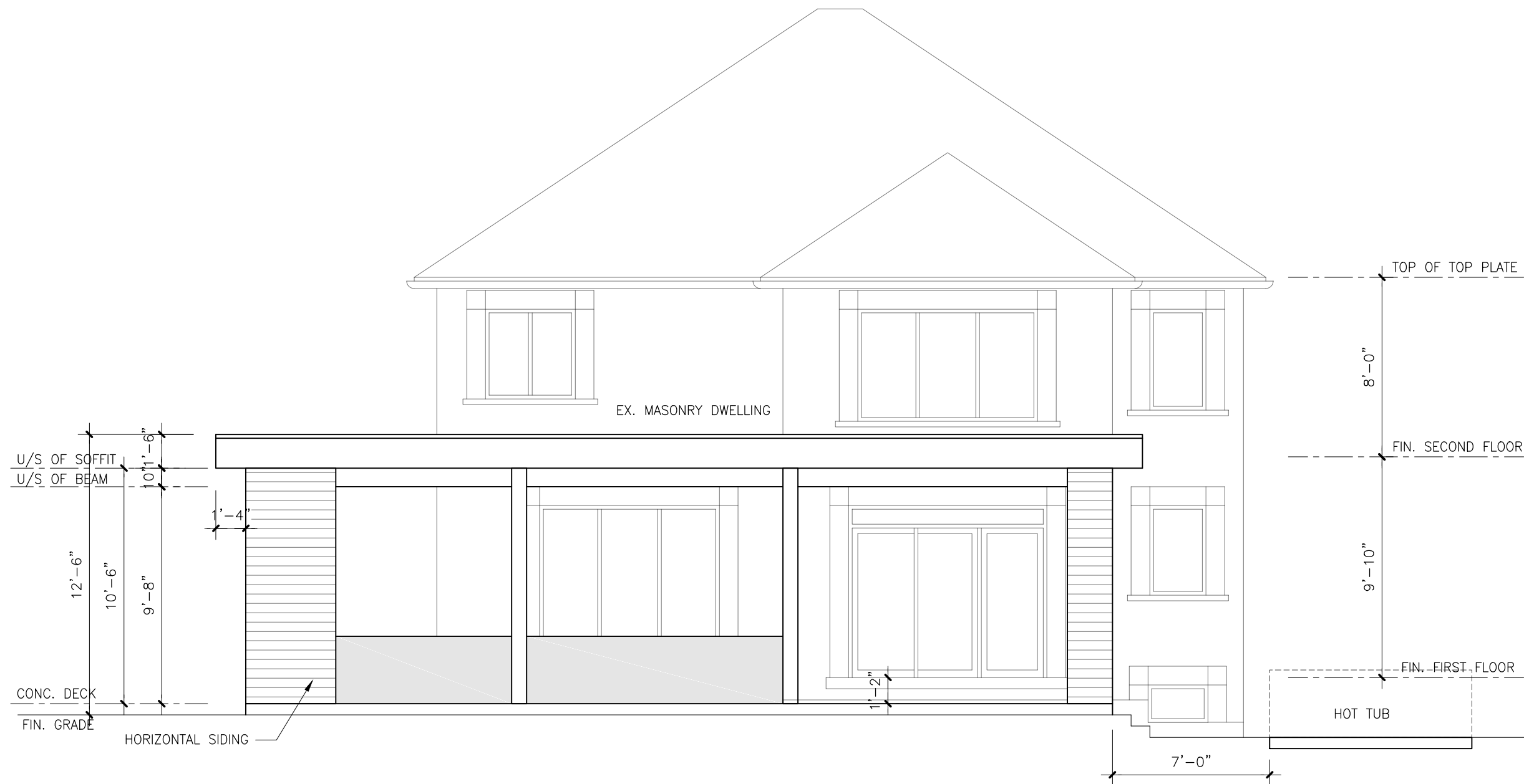
EAST ELEVATION (REAR) SCALE: 3/16" = 1'-0"
