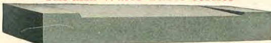
A Sill Stone made by inserting wood block in mold to form watershed.
