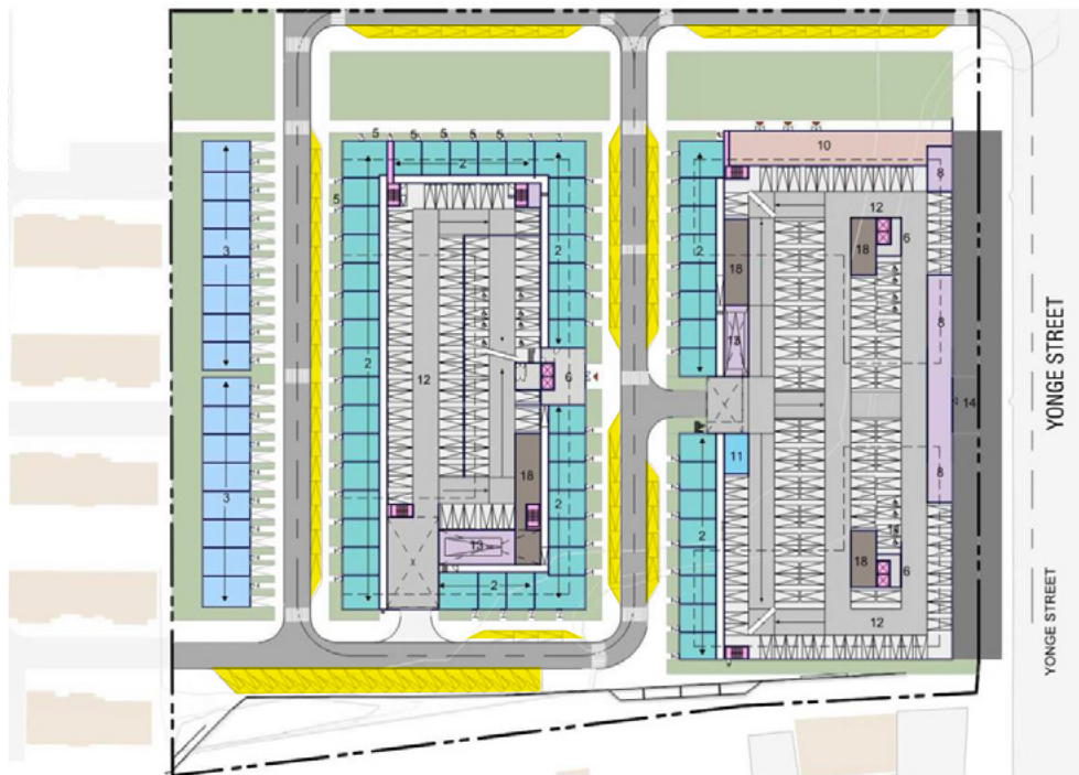
Figure 9.3 Level 1 Parking (with on-street parking in yellow)
