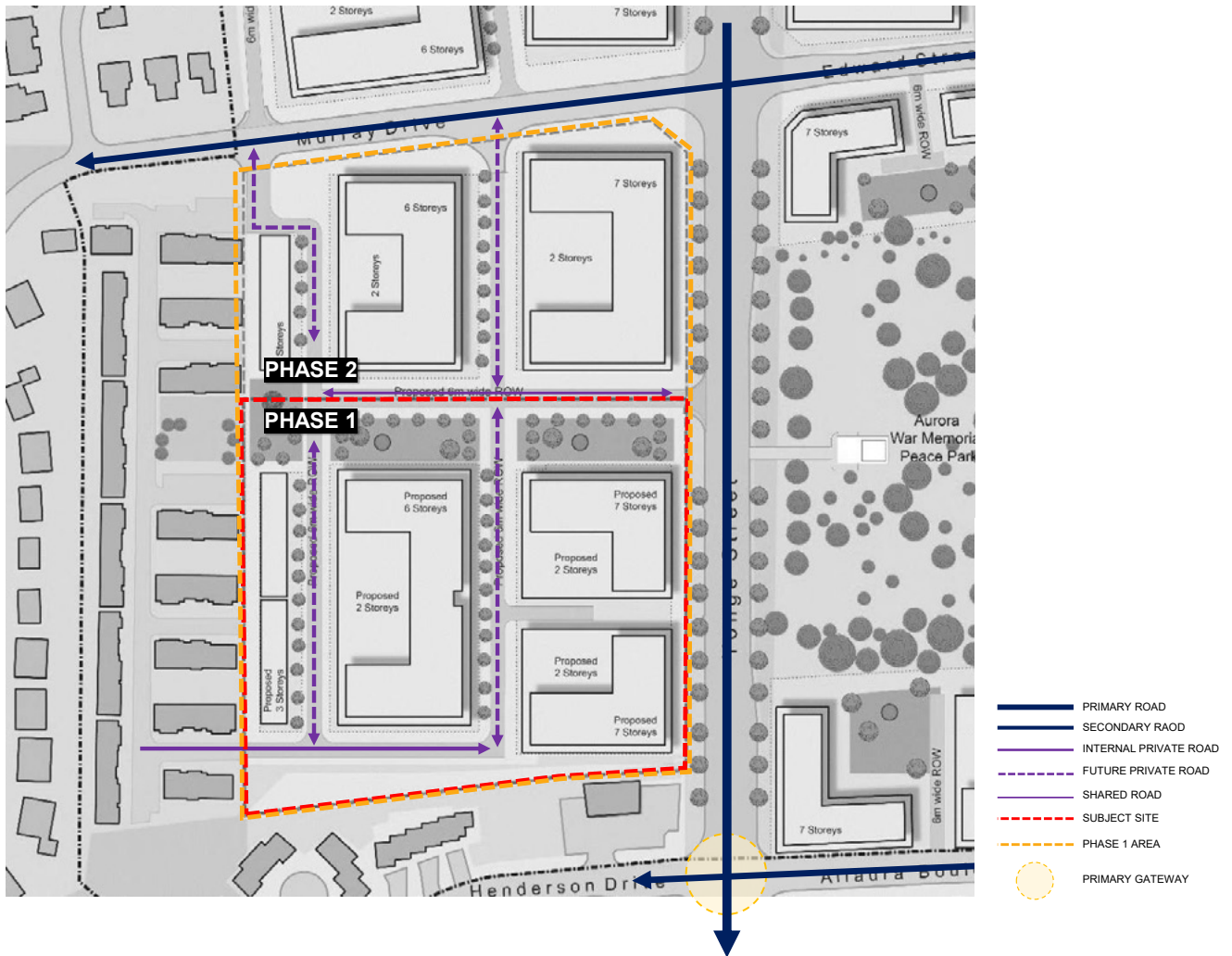
Figure 8.1 Vehicular Network across the Phase 1 Lands
